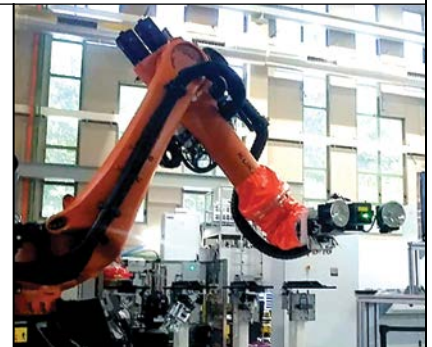
The LTI-2100, shown above, is integrated with an industrial robot for the inspection of large aerospace structures.
